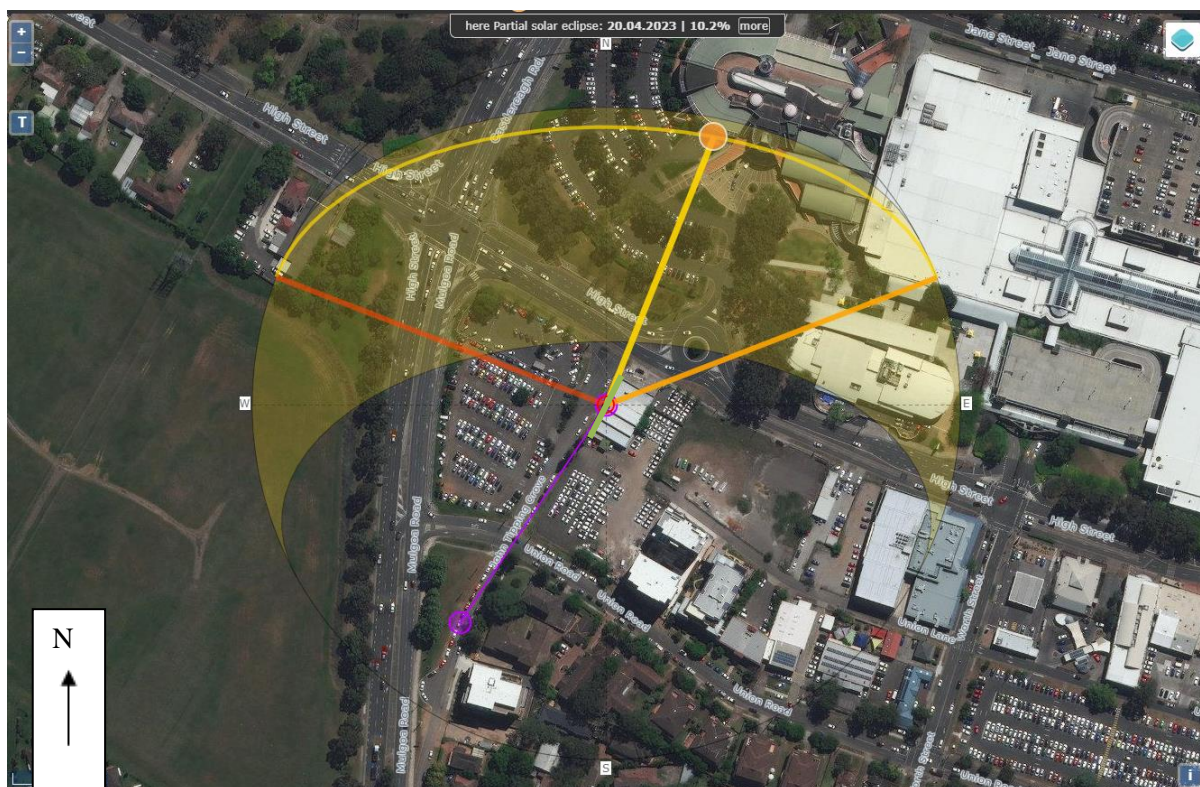
Figure 25: Representation of incident and reflection of solar rays from the S2T2's North-West façade onto John Tipping Grove.
