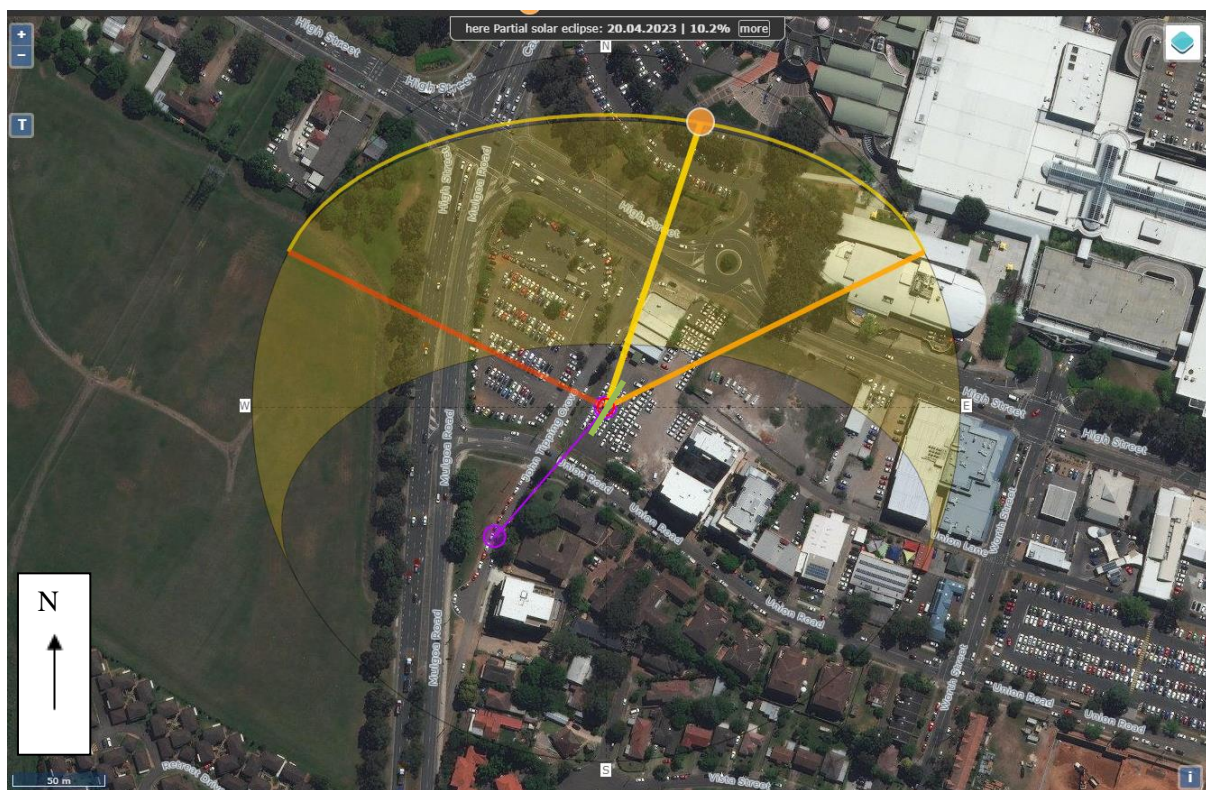
Figure 18: Representation of incident and reflection of solar rays from the S1T1's North-West façade onto John Tipping Grove.
