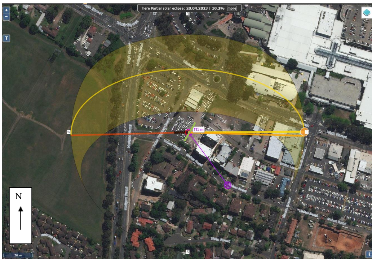
Figure 11: Representation of incident and reflection of solar rays from the Podium's South-East façade 1 onto Union Road.
