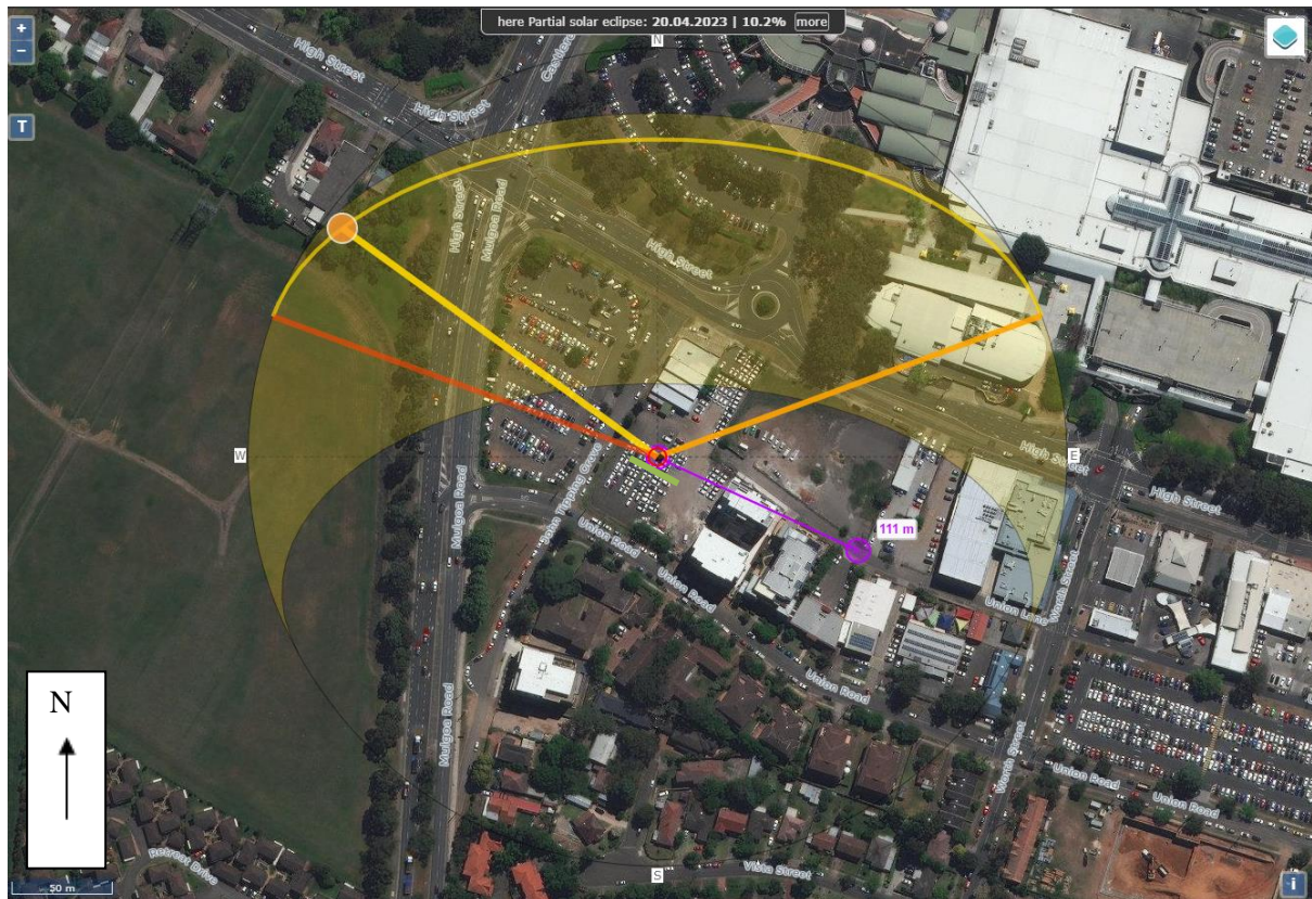
Figure 16: Representation of incident and reflection of solar rays from the S1T1's North-East façade onto Union Lane.
