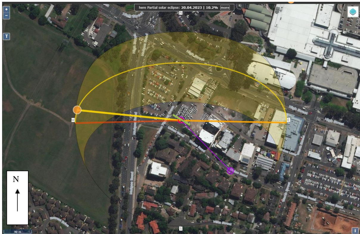
Figure 10: Representation of incident and reflection of solar rays from the Podium's South-West façade onto Union Road.
