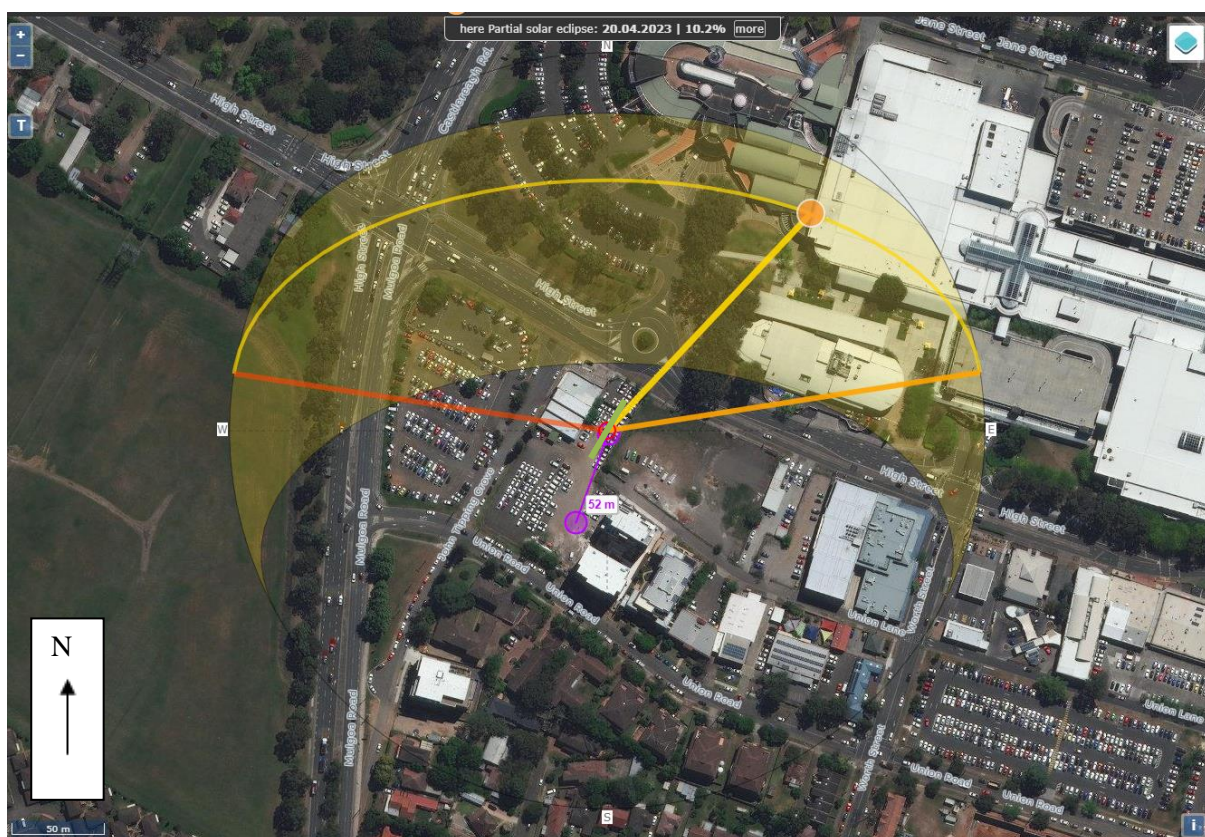
Figure 30: Representation of incident and reflection of solar rays from the S2T2's South-East façade onto Temporary New Road.
