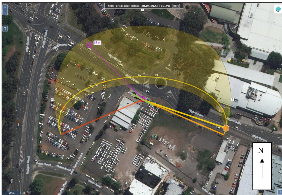
Figure 7: Representation of incident and reflection of solar rays from the Podium's North-East façade onto High Street.
