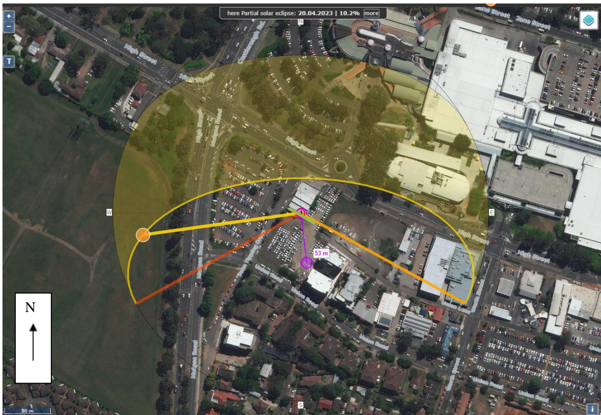
Figure 28: Representation of incident and reflection of solar rays from the S2T2's South-West façade onto Temporary New Road.
