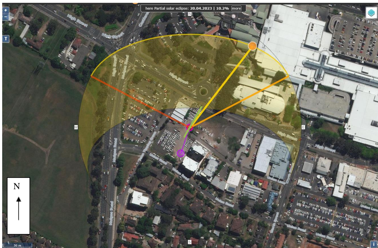
Figure 15: Representation of incident and reflection of solar rays from the Podium's South-East façade 2 onto Temporary New Road.
