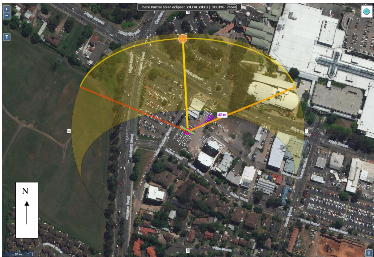
Figure 17: Representation of incident and reflection of solar rays from the S1T1's North-East façade onto Temporary New Road.
