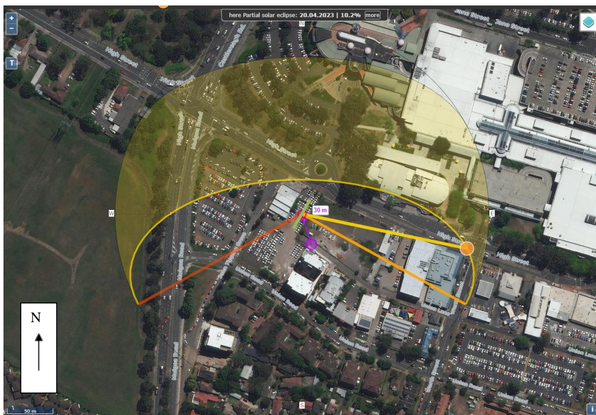
Figure 29: Representation of incident and reflection of solar rays from the S2T2's South-East façade onto Union Lane.
