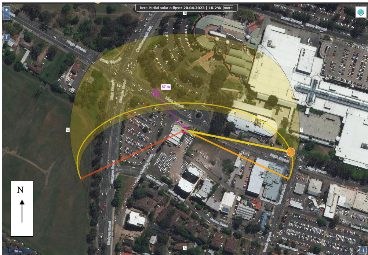
Figure 23: Representation of incident and reflection of solar rays from the S2T2's North-East façade onto High Street.
