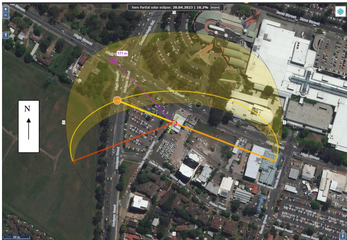
Figure 24: Representation of incident and reflection of solar rays from the S2T2's North-West façade onto High Street.
