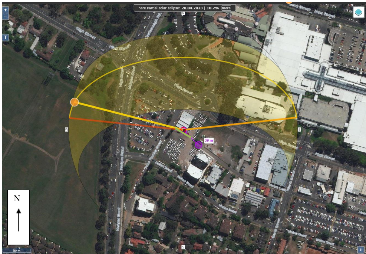
Figure 27: Representation of incident and reflection of solar rays from the S2T2's South-West façade onto Union Lane.
