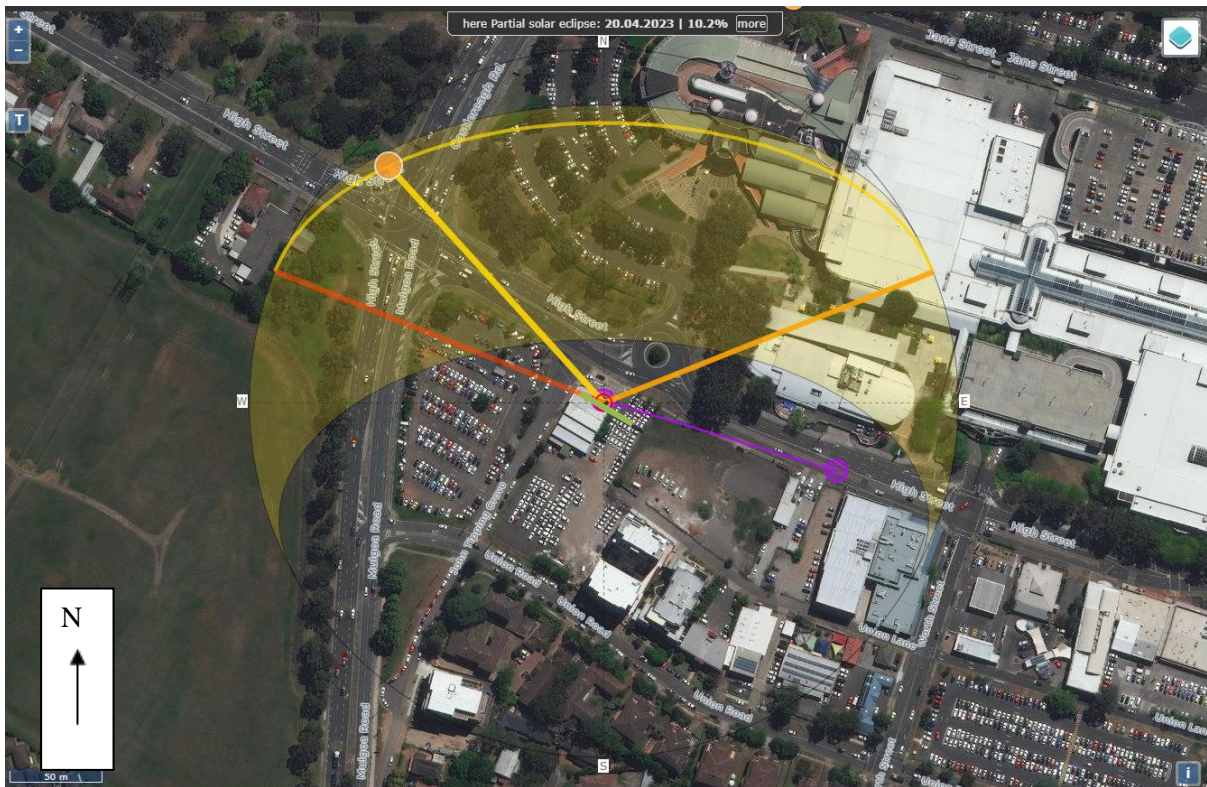
Figure 22: Representation of incident and reflection of solar rays from the S2T2's North-East façade onto High Street.
