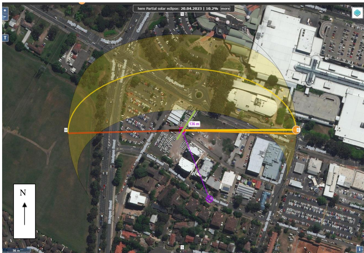
Figure 13: Representation of incident and reflection of solar rays from the Podium's South-East façade 2 onto Union Road.
