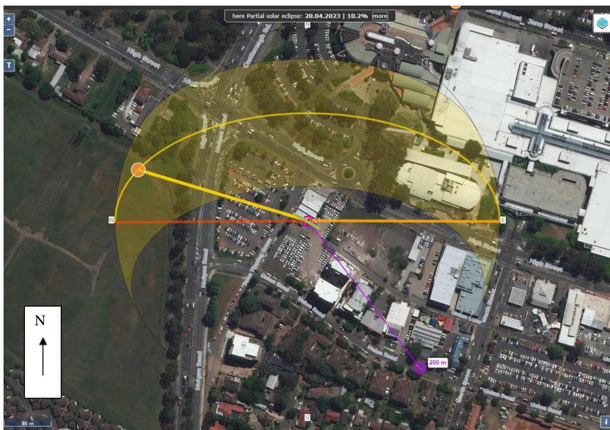
Figure 26: Representation of incident and reflection of solar rays from the S2T2's South-West façade onto Union Road.
