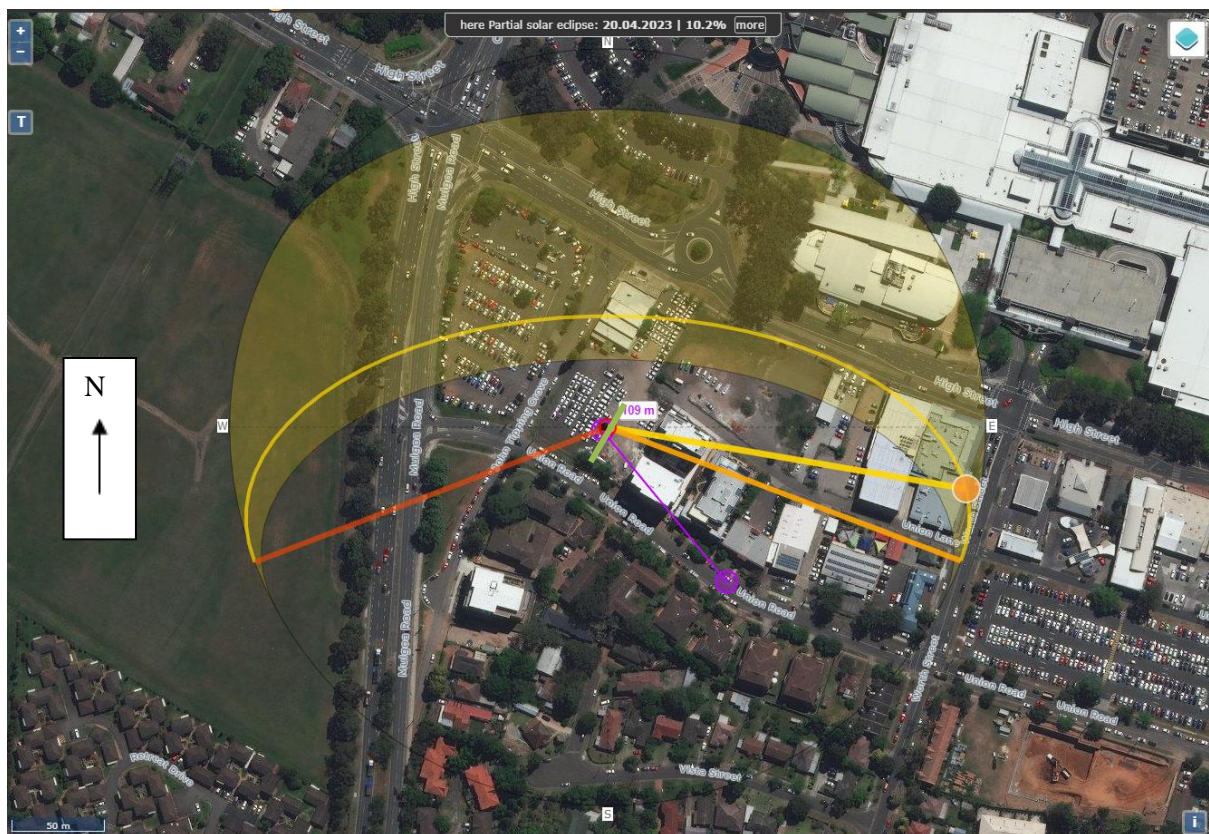
Figure 21: Representation of incident and reflection of solar rays from the S1T1's South-East façade onto Union Road.
