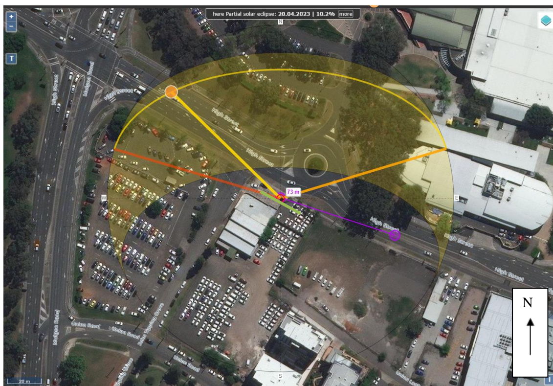
Figure 6: Representation of incident and reflection of solar rays from the Podium's North-East façade onto High Street.
